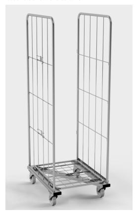
**Technical data:** structural stability is ensured by closed profiles, meshes made of steel bars, bottom with wheels (two fixed wheels, two swivel wheels), bottom shelf reinforced with flat bars. The construction enables container folding and nesting of folded containers. Standard version has chassis on wheels and two side walls.
