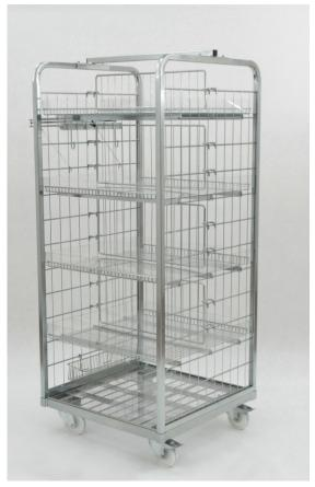
Container allows for presentation of commodities. The construction of the container is folded and bolted. The supporting construction is made of a section bar, shelves made of wire reinforced with flat bars. The possibility of height adjustment of the shelves position within the container. Shelves and base lined with Plexiglas to protect it from falling out of small products. Swivel castors, including 2 pcs. with brake. Optional accessories: basket for code reader and a holder for plastic bags.
