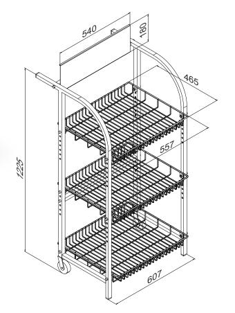
**Standard finish:** powder coated. **Technical data:** The frame is made of section, wire shelves bolted to the frame, possibility of adjust the height of the shelves on the required level. Two wheels attached to the rear legs make it easy to move the rack.
