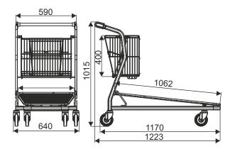
In the standard version shopping trolley has standard wheels. Optional accessories (inter alia wheels for travelator or with brake, coin lock, logo and other accessories) require separate arrangements.
