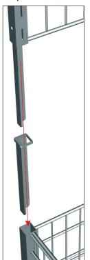
Adapter to overhead attachment from section 30x30x2
