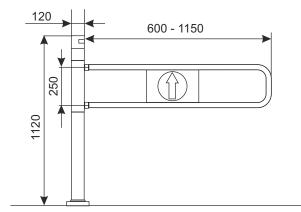
An electronic gate Porta'e RADAR is steering by radar without lighting. Gate can be available in two option: right or left - opens in right side or left side. The gate opens automatically in the direction of entry as you approach it. The gate closes also automatically.
